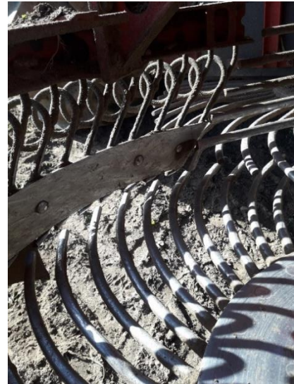
Photo: Use of bar gates/plates to minimise damage and losses.
