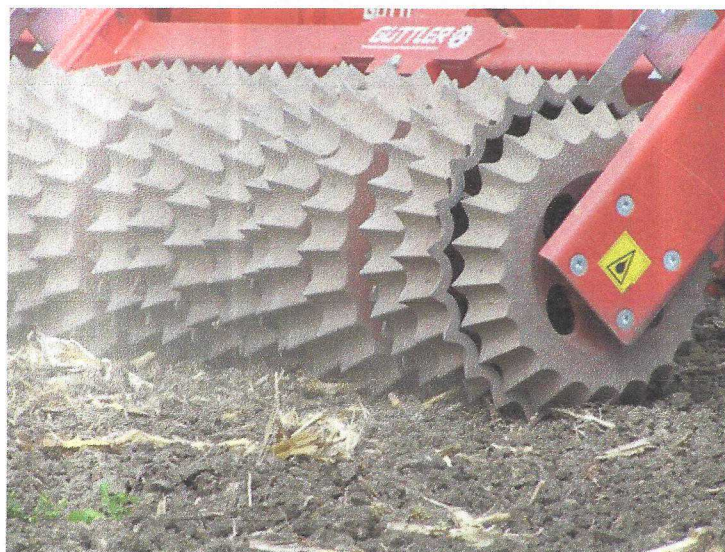
Figure 12: The use of a prism roller can assist in producing a suitable tilth.
