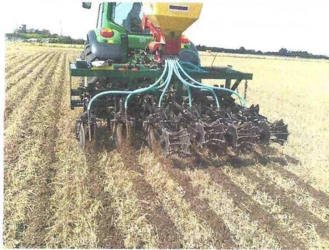
Figure 2: Strip tillage cultivation creating a defined cultivated zone.
