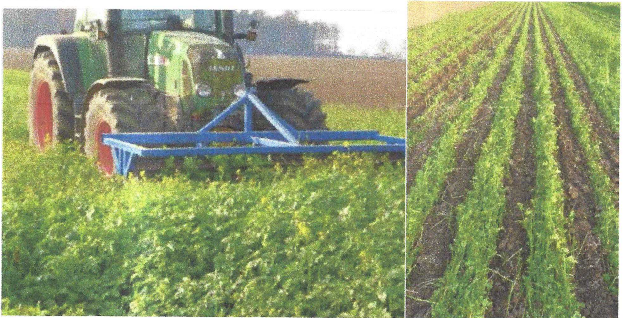
Figure 18: Using a front mounted flail in a mustard cover crop prior to cultivation using strip tillage (Pflugfelder, 2014).
