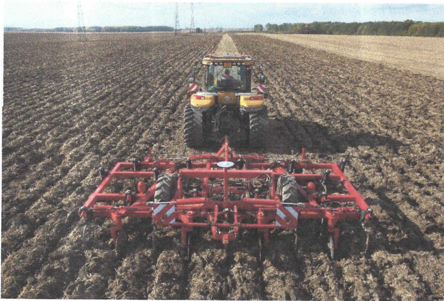
Figure 6: Ridge tillage in autumn to produce a rough seedbed prior to weathering (Image courtesy of Michael Horsch).
