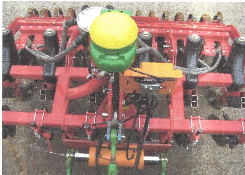
Figure 4: RTK implement shifting using hydraulic adjustment.
