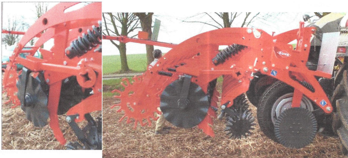
Figure 11: Kuhn Striger strip tillage implement fitted with winged tines and wavy discs to produce the seedbed and finger tines at the rear to provide consolidation (Roisin, 2014).
