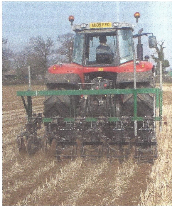
Figure 10: Yetter strip tillage implement fitted with rolling baskets to improve seedbed tilth.
