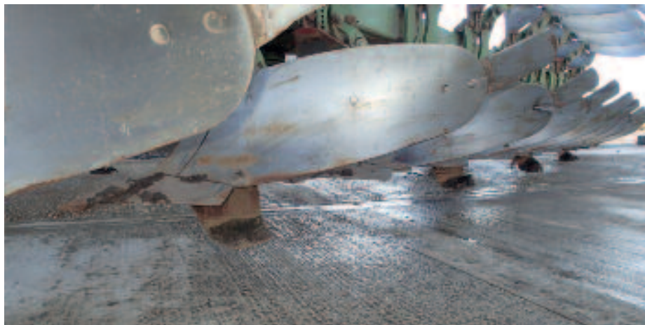
Pic. 2 – Loosener units fitted below the plough bodies.
