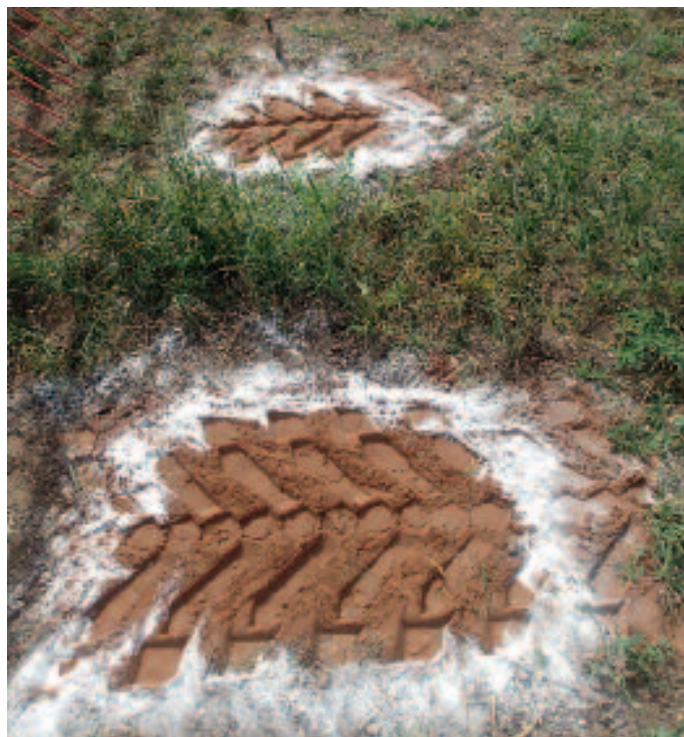
Pic. 4 – VF tyre contact patch at low pressure (foreground) and conventional pressure (background) on same axle.
