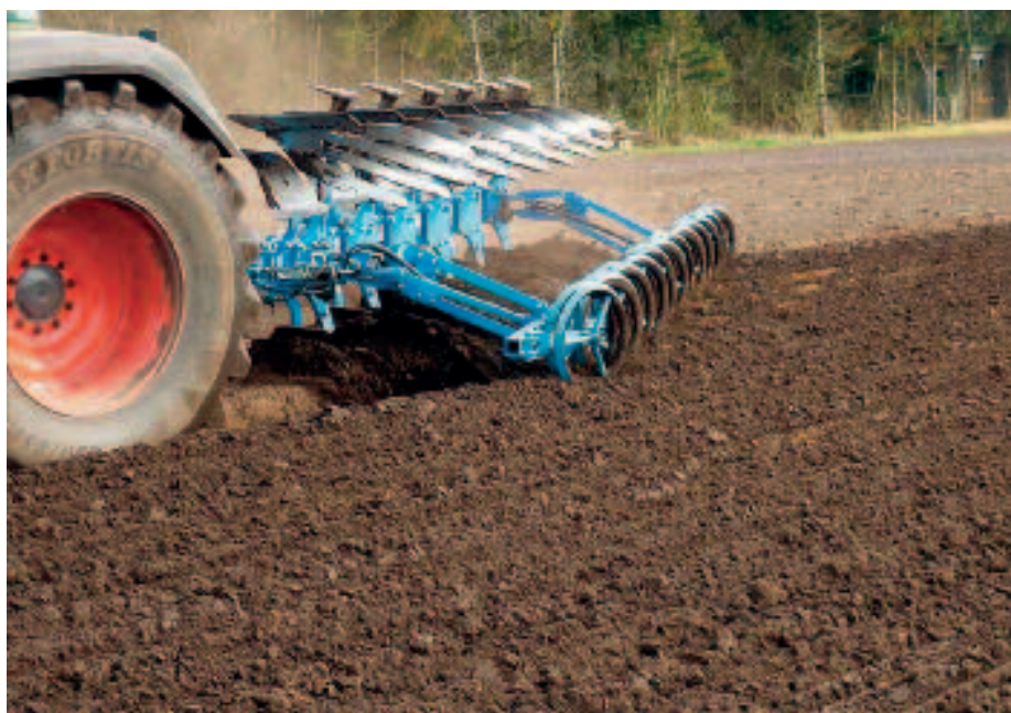
Pic. 3 – Integral plough and press for lighter soils,
