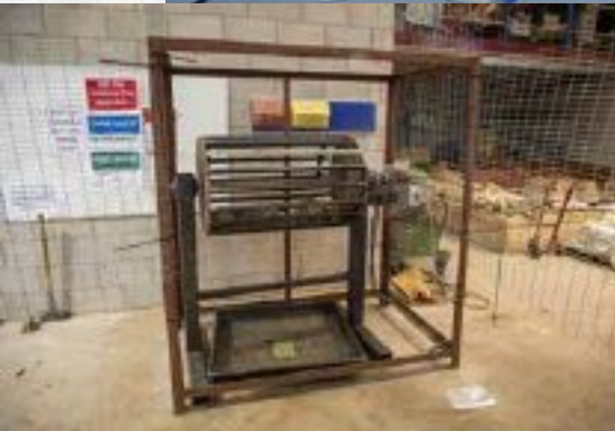
Fig. 3. Sugar beet basher used to damage sugar beet roots.
