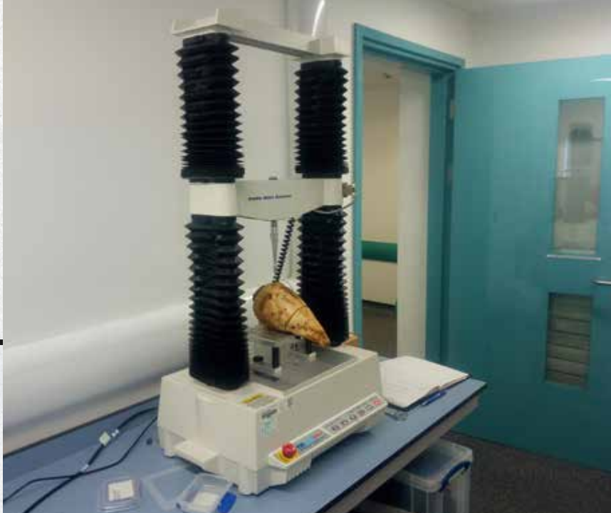
Fig. 2. A textural analyser TA.HDplus - Stable Micro systems Texture analyser, (Godalming UK) used to analyse root tissues.
