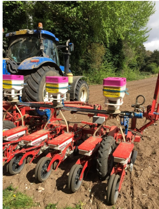
Fig 2: Granule applicators such as those pictured on this drill will soon be dispensing garlic-based NEMguard DE instead of synthetic nematicides, after nearly 50 years of use protecting sugar beet from FLN.
