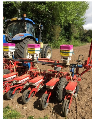
Fig 2: Granule applicators such as those pictured on this drill will soon be dispensing garlic-based NEMguard DE instead of synthetic nematicides, after nearly 50 years of use protecting sugar beet from FLN.
