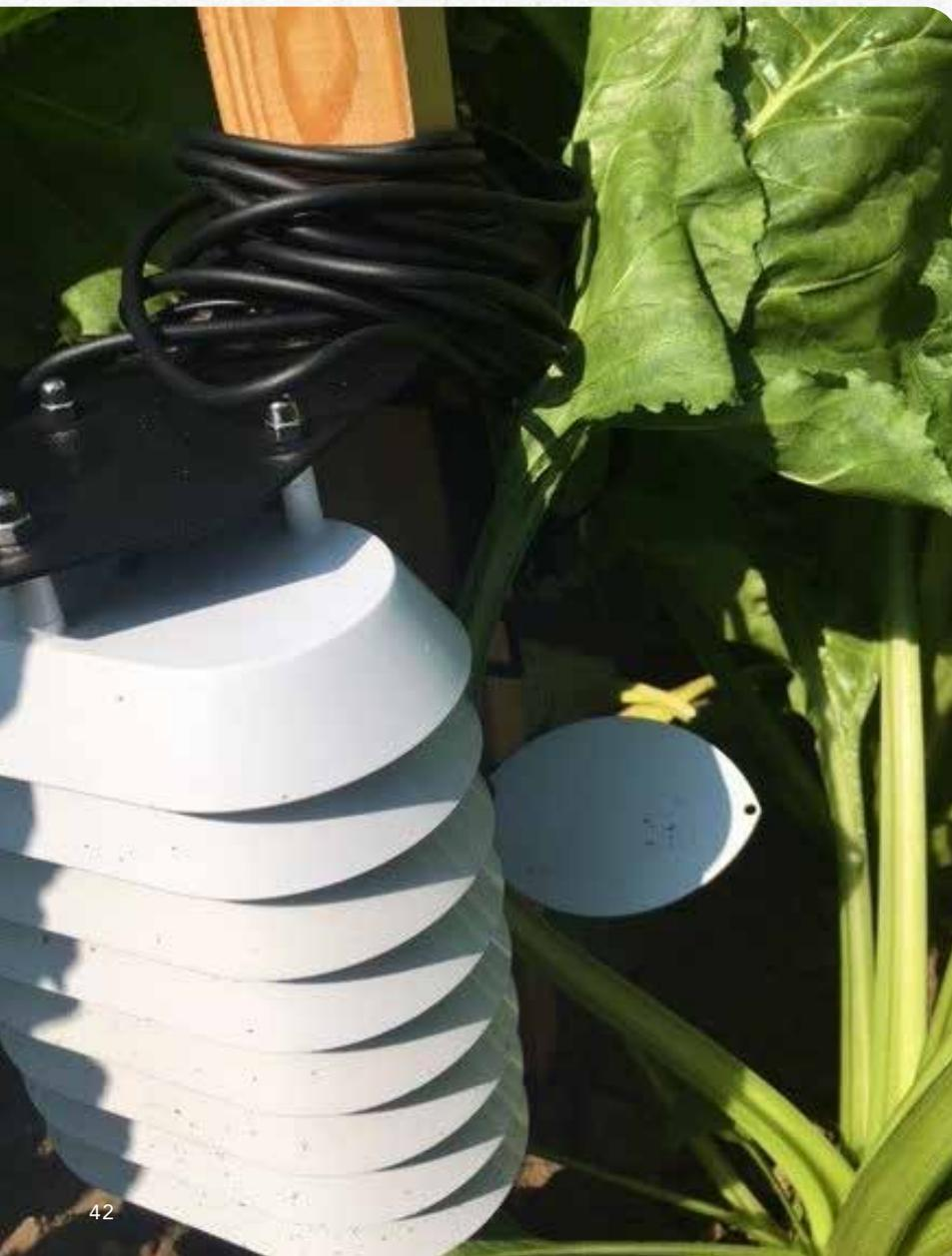
**Fig. 11.** Sencrop sensor detecting leaf wetness
