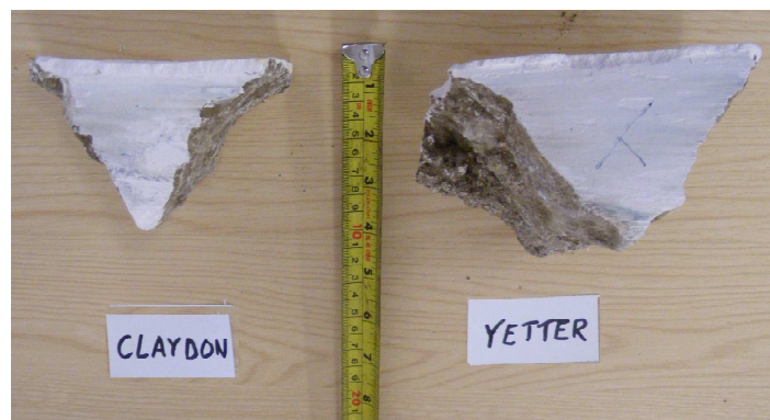
Figure 3: Comparison of a Yetter strip tillage implement with a Claydon drill and the area of soil disturbed as indicated by plaster casts.
